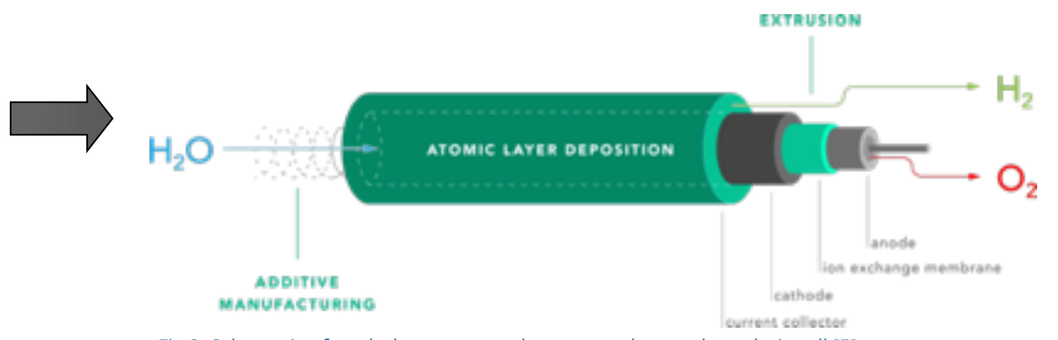
Fig 2: Schematic of a tubular proton exchange membrane electrolysis cell [5]
