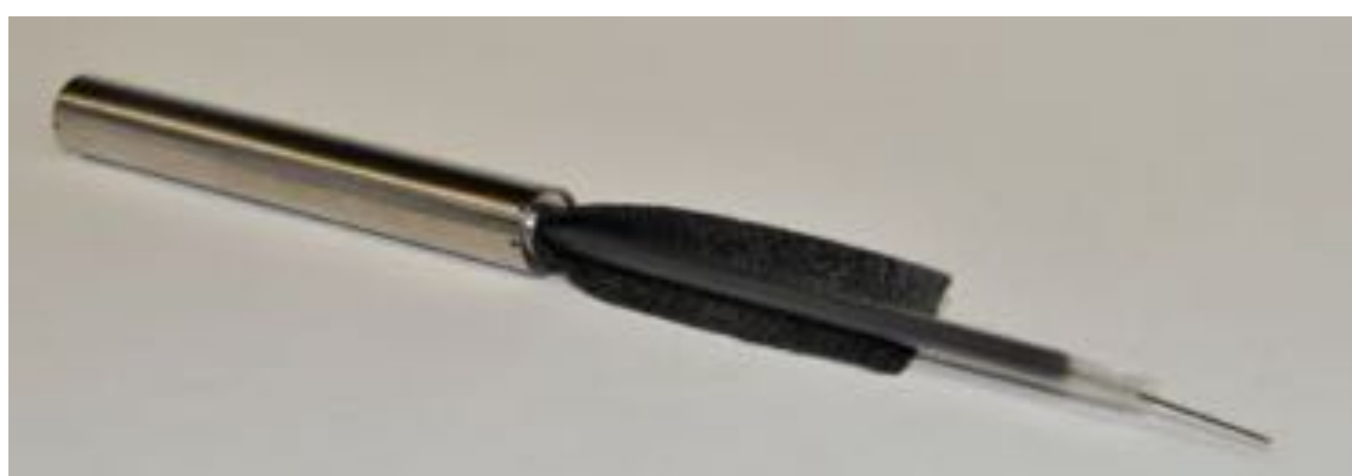
Fig 4: Fabrication of a tubular PEM electrolysis cell
