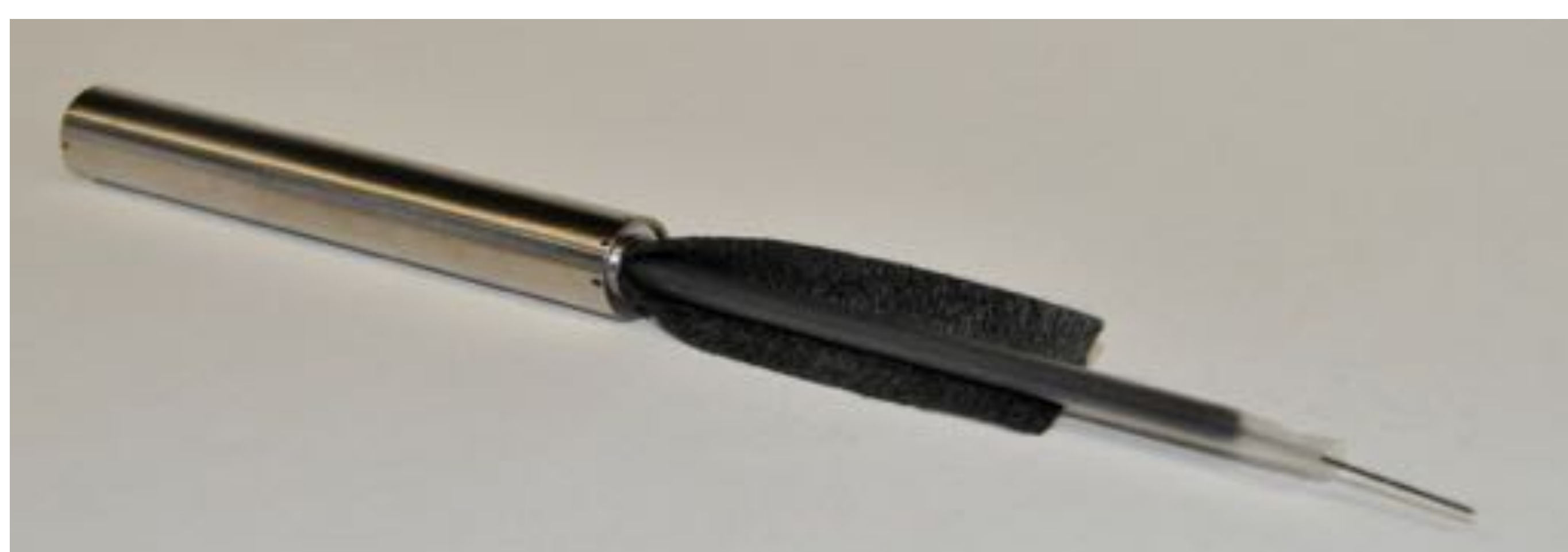
Fig 4: Fabrication of a tubular PEM electrolysis cell
