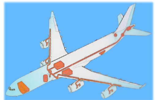
Air distribution system in an aircraft
